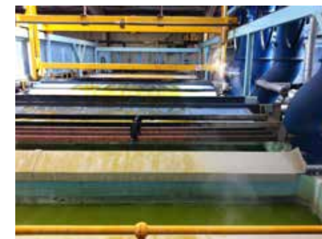
Oxidising the Sheets to Add the Colour
